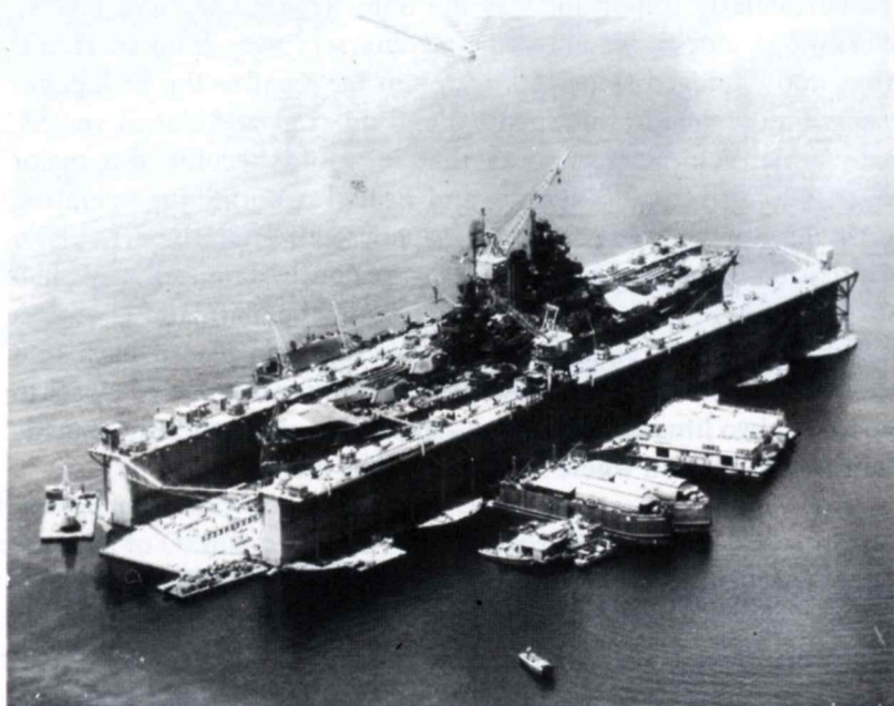
Fig. 10. The battleship USS Mississippi in the ABSD-5 floating drydock off Manicani Island.
